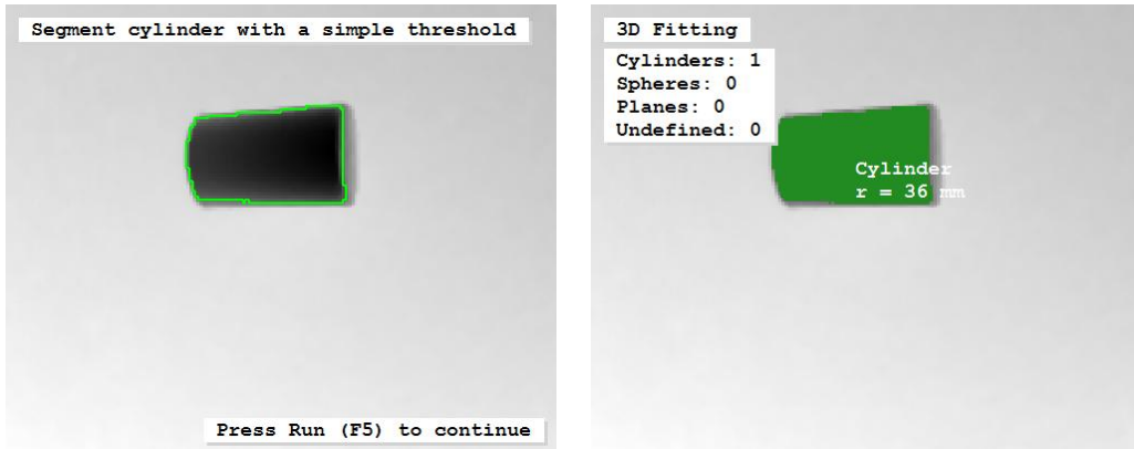
Figure 4.14: 3D primitives fitting: (left) simple threshold for 2D segmentation, (right) result returned by the fitting.
