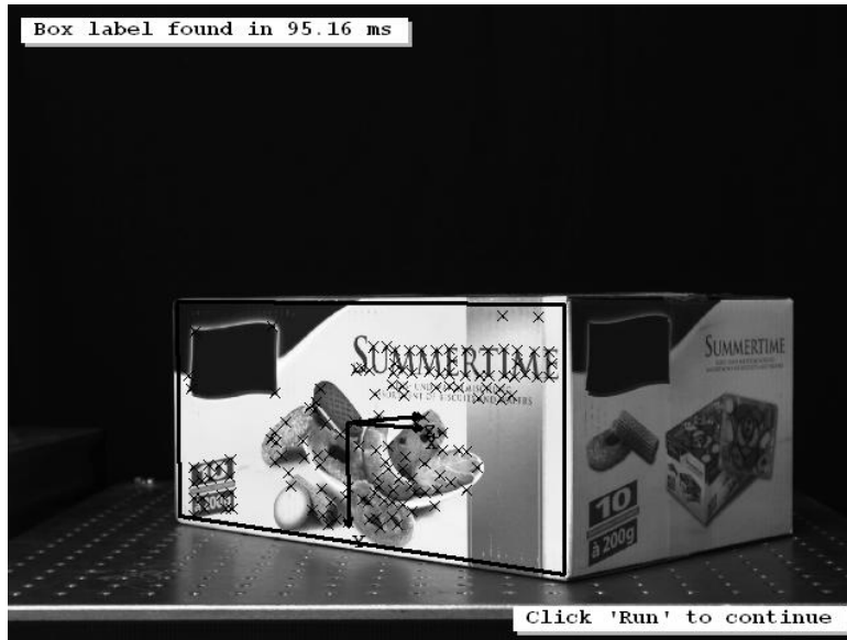
Figure 4.17: 3D pose of a cookie box label obtained by a calibrated descriptor-based matching.
