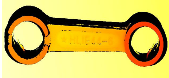
Figure 6.13: Result of uncalibrated sheet-of-light measurement: disparity image.
