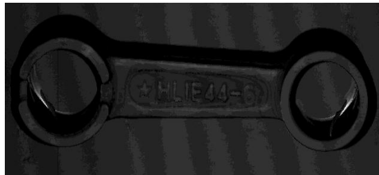
Figure 6.15: Result of uncalibrated sheet-of-light measurement: score image (score_type set to 'width', i.e., bright parts indicate artifacts).
