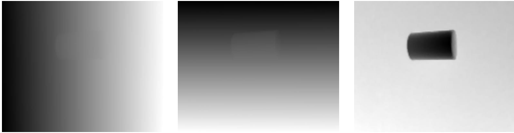
Figure 4.13: Height data used for 3D primitives fitting: (from left to right) X, Y, and Z image.
